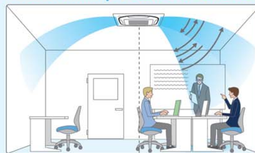
Optimal air direction by "Auto" Swing (narrow)
